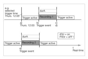
Only possible for trigger types triG = in and triG = out. The pre-trigger must be deactivated in this mode (PrEtr = oFF)!
